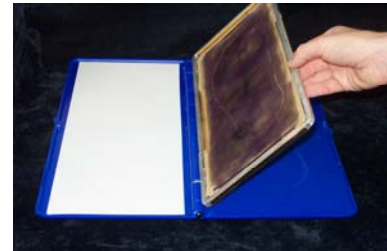
Fig. 3 – Insert paper onto the blue cover opposite the inked rubber mat and flip over so the crosshatched side is face down on the paper.
