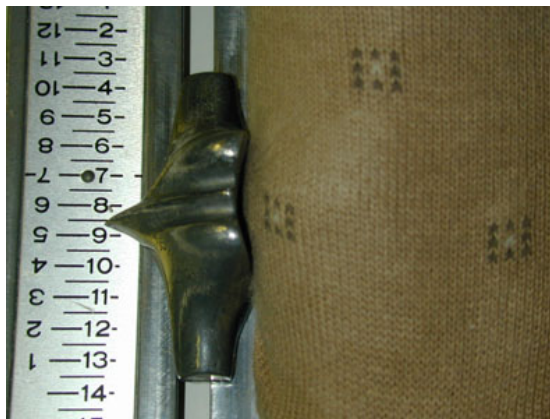
Fig. 8 - In the photo (right), the heel to ball measurement should be recorded as an 8½ +.
