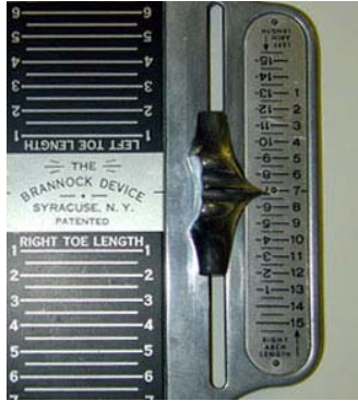
Fig. 2 - Movable Arch Length Pointer
