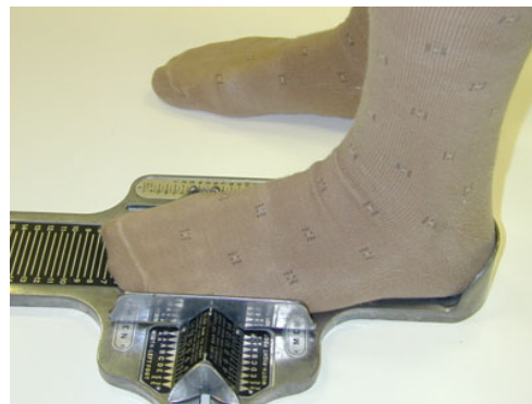
Fig. 5 – Lateral view of proper foot placement in the Brannock Device
